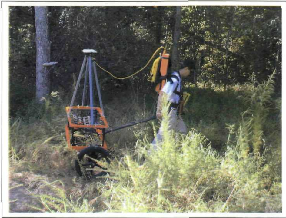
Photograph #1 – EM61/GPS Geophysical Survey in Progress – Single Cart EM61 Manual Configuration.
